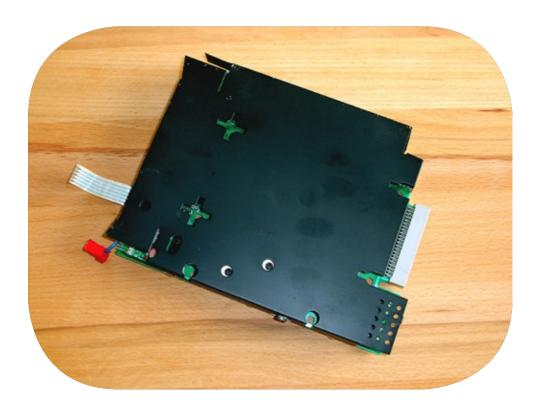
Gently push the knife between the main board and the shielding and lever the blade down a bit as shown in the photo. Break the soldering point with the soldering iron. Proceed until all soldering points have been desoldered. Check whether the small metal plate of the reset button is still in place. It tends to fall off...
