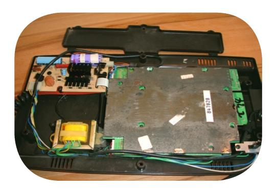
Locate the power supply unit and detach the white and the blue cable at the right side of the board. Be sure to memorize polarity of the white cable.
