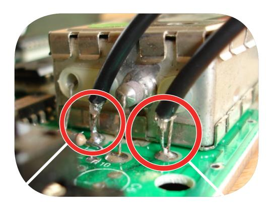
When the cables are correctly soldered to the RF section put the shielding back in place.
