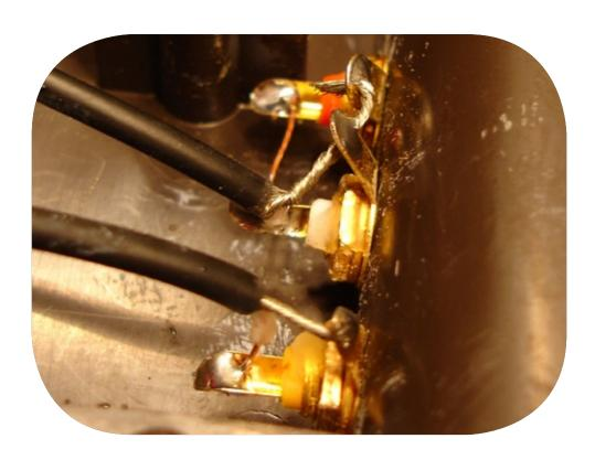
Put the main board back into the casing, connect the hand controllers to it (POLARITY!) and the blue wire to the power supply PCB. Solder the red wire ,+5 V'' from the mod to the white power cable like shown in the picture. Choose the topmost connector and do not damage the other conducting paths! Be extra careful when you put the soldering wire to the white cable, it can melt when it is overheated. Connect the white power cable to it's jack on the power supply PCB, ensuring correct polarity.
