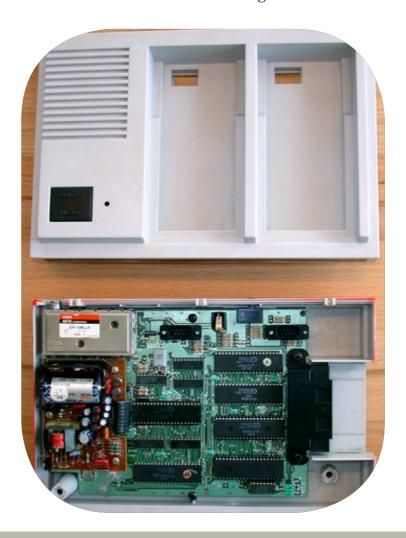
Locate the power supply and unscrew all three screws. Turn the PCB upside down.
