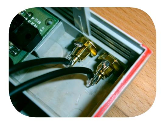
Place the cables under the Intv PCB and put the the Intv PCB back inside the chassis. Place the mod board in the open area next to the composite connectors. Tighten the four screws that hold the Intv PCB down.
