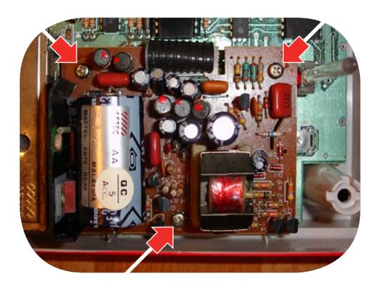
Solder the red wire "+5V" from the mod to the power supply PCB as shown in the picture. You should attach the wire to the third soldering point to the left of the notch. The correct soldering point is wider than the others:
